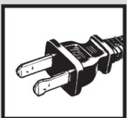
**THIS APPLIANCE HAS A POLARIZED PLUG (one blade is wider than the other). To reduce the risk of electric shock, this plug is intended to fit in a polarized outlet only one way. If the plug does not fit fully in the outlet, reverse the plug. If it still does not fit, contact a qualified electrician to install the proper outlet.**
